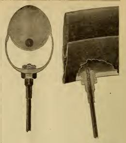
METHOD OF FASTENING SPOKES. WHICH ADMITS OF REPAIRS WITHOUT REMOVING TIRE. NOTE SOLID CORE IN RUBBER TIRE WHICH PREVENTS Our Wheels are built on the most stretching. Note elliptical shape of tire. NOTE THE THICKENED RIM ON LINE OF SPOKE HOLES; ALSO THICKENED SPOKES AT POINT MOST LIABLE TO BREAK.
