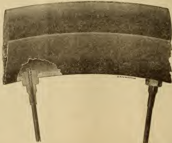
METHOD OF FASTENING SPOKES, WHICH ADMITS OF REPAIRS WITHOUT REMOVING TIRE. NOTE SOLID CORE IN RUBBER TIRE WHICH PREVENTS STRETCH. NOTE ELLIPTICAL SHAPE OF TIRE. NOTE THE THICKENED RIM ON LINE OF SPOKE HOLES; ALSO THICKENED SPOKES AT POINT MOST LIABLE TO BREAK.
