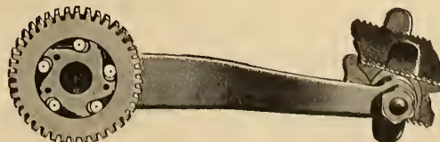
Showing Lever, Pedal, Gear, and Clutch from its Inner Side.
