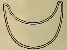
Section of front wheel felloe on Columbia Light Roadster. Actual size.
