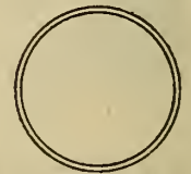
Section of rear wheel felloe on Columbia Light Roadster. Actual size.
