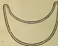
Section of front wheel felloe on Columbia Light Roadster. Actual size.
