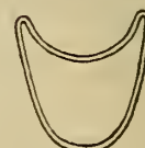
Section of front wheel felloe on Columbia Racer. Actual size.
