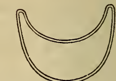
Section of front wheel felloe on Columbia Light Roadster. Actual size.
