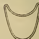
Section of front wheel felloe on Columbia Light Roadster. Actual size.
