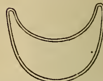
Section of front wheel felloe on Columbia Light Roadster. Actual size.
