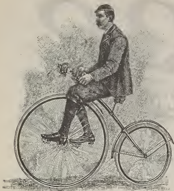
This illustration shows a man of average height on a 36 inch F. D. Safety, geared to 60 inches.
