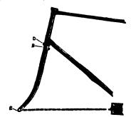
The cut represents the front fork and steering tube in position in the frame of a bicycle. A stout rod C connects the two sides of the fork. One end of the chain is securely fixed to the rod C, and the other to a block which can be slowly, but irresistibly, pulled backwards by a powerful screw.
